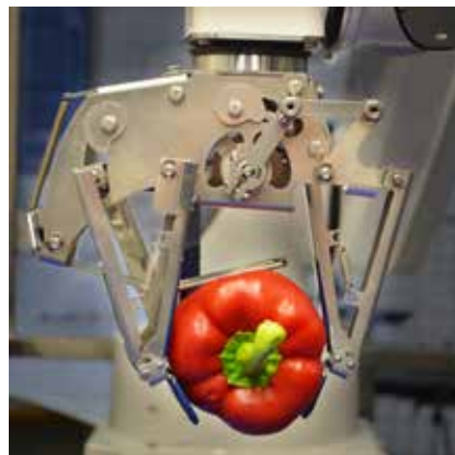
A robotic hand that can pick fruits. (Photo: Lacquey, Food Handling Solutions, Delft)
