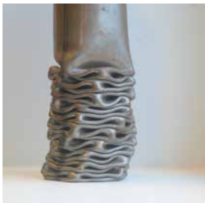
Thin-walled systems can fail spectacularly. (Photo: Jos Wassink)
